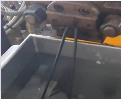
Compounding of a bioplastic composite (extruder die for two filaments (above) and water bath (below))
