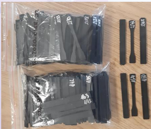
Bioplastic composite with 15 wt.% humus (lower part of the picture) and 30 wt.% of humus (upper part of the picture)
